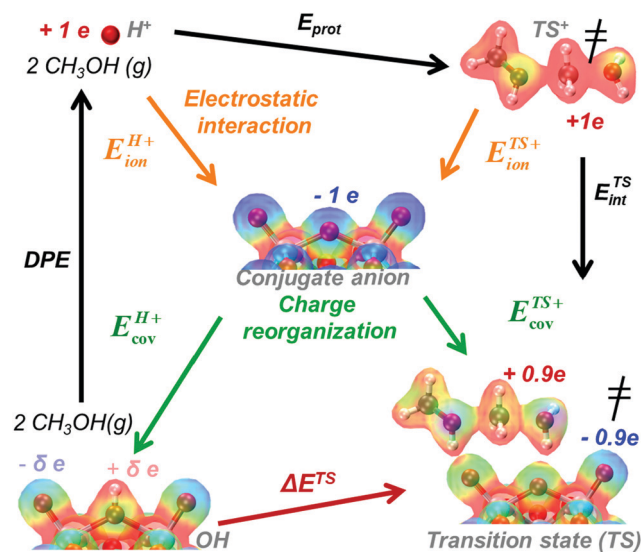
Scheme 6 The energy of DME formation transition state referenced to a bare acid and two gaseous \text{CH}_3\text{OH} molecules ( \Delta E^{\text{TS}} ) described in terms of the acid's DPE, the gas-phase protonation energy ( E_{\text{prot}} ) and interaction energy ( E_{\text{int}}^{\text{TS}^+} ) of cationic transition state analog with its conjugate anion. DPE and E_{\text{int}}^{\text{TS}^+} reflect ion-pair interactions with electrostatic (ionic) and charge reorganization (covalent) components. Colors on electron distributions reflect electrostatic potentials (red = positive, electron deficient; blue = negative, electron rich). Adapted from results and methods in ref. 33.
