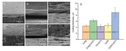
Fig. 3 SEM images of cross-sections of bare Ti (A) and coated Ti: Ti-Alq (B), Ti-Alq-CaCO<sub>3</sub> (C), Ti-CaCO<sub>3</sub> (D), Ti-DS (E), and Ti-DS-CaCO<sub>3</sub> (F); the average thickness of these coatings (G).
