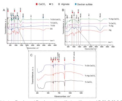
Fig. 4 ATR-FTIR spectra of the bare Ti surface and Ti surfaces with modifications: (A) spectra of Ti-DS, Ti-DS-CaCO<sub>x</sub>, Ti-CaCO<sub>x</sub> and dextran sulfate powder; (B) spectra of Ti-Alg, Ti-Alg-CaCO<sub>3</sub>, Ti-CaCO<sub>3</sub> and Ca<sup>2+</sup>-crosslinked Alg hydrogel; and (C) spectra of mineralized Ti surfaces (Ti-CaCO<sub>3</sub>, Ti-Alg-CaCO<sub>3</sub>, Ti-DS-CaCO<sub>3</sub>) in the wavenumber range 250–1300 cm<sup>-1</sup>.
