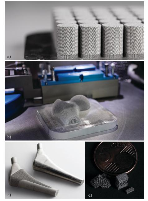
Fig. 1 A number of AM porous metallic biomaterials including the cylindrical specimens used for mechanical testing (a), a functionally graded porous structure in the shape of the femur with different porosities (b), hip stems with external and internal porous structures (c), and multiple miniaturized porous specimens (d). Most specimens are designed and fabricated from the titanium alloy Ti-6Al-4V at the Additive Manufacturing Lab (TU Delft)
