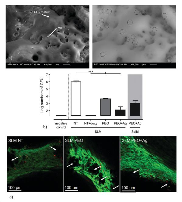
Fig. 10 Silver nanoparticles immobilized on the surface of AM porous metallic biomaterials using plasma electrolytic oxidation minimize the risk of implant-associated infections (a). In an ex vivo test, the number of bacteria could be decreased by  $\approx 4$  orders of magnitude (b). Interestingly, cell viability even increased in comparison with a non-treated porous specimen<sup>145</sup> (c).
