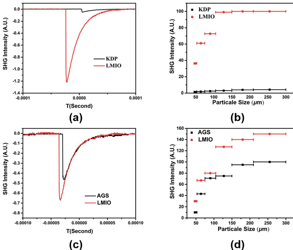
Fig. 4 Oscilloscope traces of the SHG signal (150–210 nm) of LMIO at (a) 1064 nm and (c) 2.05  $\mu\text{m}$ . Plots of measured SHG intensity vs. particle size of LMIO under laser radiation at (b) 1064 nm and (d) 2.05  $\mu\text{m}$ . KDP and AGS samples serve as the references for 1064 and 2.05  $\mu\text{m}$  laser radiation, respectively.
