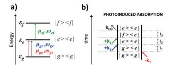
Fig. 4 (a) Scheme of the three-level system, showing transition dipole moments ( $\mu$ ) and frequencies ( $\omega$ ) associated with the ground (g) and excited (e,f) states and their energies ( $\varepsilon_{g,e,f}$ ). (b) Feynman diagram of a PA signal.
