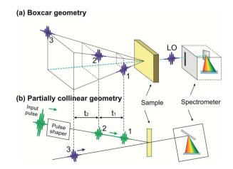
Fig. 3 The experimental configurations used for 2D spectroscopy: the non-collinear 3PPE (a) and the partially collinear PP geometry (b).
