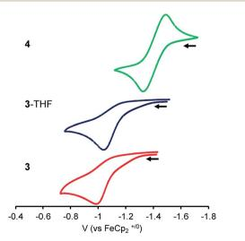
Fig. 3 CVs of 3, 3-THF and 4 with 0.1 M  $[^nPr_4N][BAr_4^F]$  electrolyte in DFB (scan rate of 100 mV s<sup>-1</sup>; collected under Ar).
