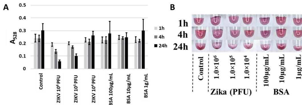
Fig. 8 Best performing aptamer, CFA0204, detecting Zika virus. (A) ZIKV at  $10^5$  PFU was able to induce aggregation as evidenced by a decrease in  $A_{528}$ . (B) While precipitation was apparent, no shift to a blue color was induced by ZIKV.
