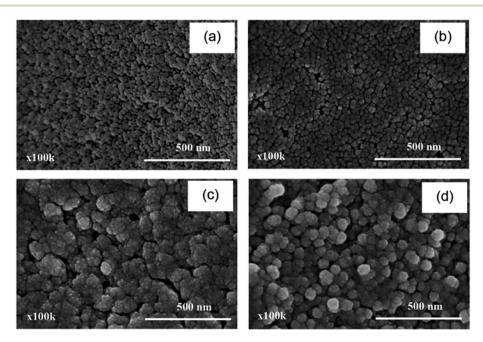
Fig. 6 PEDOT: PSS surface morphology at the EDOT: PSS weight ratio of 1: 11 and EDOT:  $Na_2S_2O_8$  mole ratio of 1: 2 using various surfactant types: (a) no surfactant, (b) CTAB (2.5CMC), (c) SDS (2.5CMC), and (d) Triton X-100 (2.5CMC).
