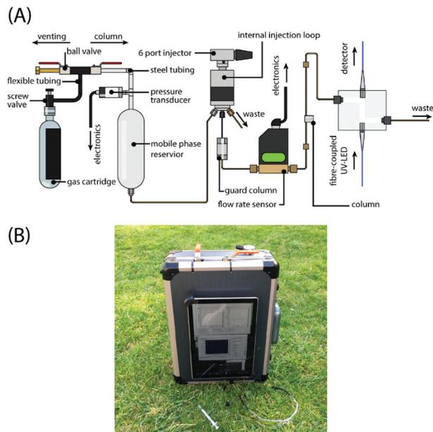
**Fig. 1** Portable high-performance liquid chromatography. (A) The schematic shows the key system components and their connectivity. The components are depicted for clarity and are not intended to dictate an orientation of operation. (B) Photograph of the ‘chromatography in a suitcase’ system running separations in the field.
