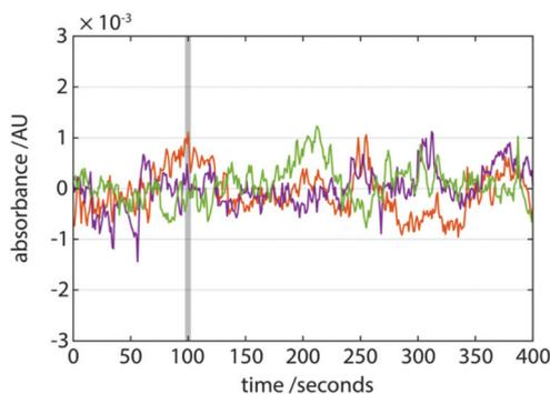
**Fig. 4** Mechanical stability of the device is tested by repeated 1 m drop tests. Traces ( $n = 3$ ) show the baseline absorbance before and after impact. The grey vertical bar indicates the approximate time at which the device is released and impacts the floor. No change in baseline absorbance mean or variance is observed as a result of the drop tests.
