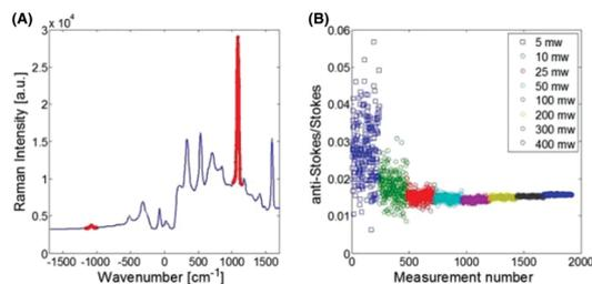
**Fig. 1** (A) Raman spectrum of Au-MBA nanoparticles alone deposited on CaF<sub>2</sub> with the (1085 cm<sup>-1</sup>  $\nu_{12}$  benzene ring mode) highlighted in red. (B) anti-Stokes/Stokes intensity ratio ( $\nu_{12}$  benzene ring mode) of MBA labelled gold nanoparticles alone deposited on CaF<sub>2</sub> measured between 5–400 mW at 830 nm excitation.
