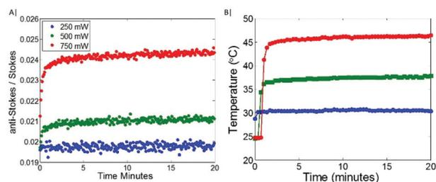
**Fig. 2** (A) Anti-Stokes/Stokes intensity ratio of the 1085 cm<sup>-1</sup>  $\nu_{12}$  benzene ring mode of Au-MBA labelled nanoparticles co-localised with NIR absorbing Au-NS deposited on CaF<sub>2</sub>, under different illumination powers (250, 500 and 750 mW) at 830 nm excitation. (B) Peak temperature of the Au-MBA and Au-NS while illuminated with 830 nm laser beam under different laser powers (blue 250 mW, green 500 mW and red 750 mW) measured by thermal imaging camera.
