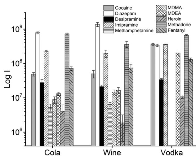
Fig. 6 TFME-DBDI-MS ion signals for fast extractions ( $n = 3, 5$  seconds) of beverages (1.5 mL) spiked with a mix of drugs at  $1 \mu\text{g mL}^{-1}$ . No agitation of the sample was performed. A quick (3 s) rinse of the TFME device by immersion in LC-MS grade water was performed prior to thermal desorption and DBDI-MS analysis. Each extracted ion chromatogram was integrated for 0.5 min.
