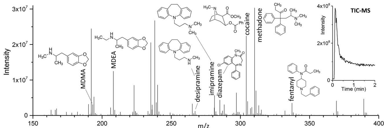
Fig. 2 Direct TFME-DBDI full scan mass spectrum of a 10 ng mL<sup>-1</sup> mix of drugs in blood plasma (containing 1% ACN), extracted for 5 minutes with ultrasound. The data shows the simultaneous ionization of the compounds and the low level of background signals. On the top right corner, the TIC for the desorption (260 °C) is shown.
