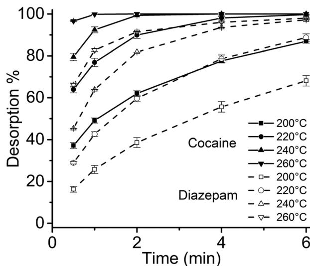
Fig. 3 SPME-DBDI-MS desorption time profiles of cocaine and diazepam at different temperatures (200 to 260 °C) for the 3 × 20 mm thin film microextraction device ( $n = 3$ ). A 4 mm I.D. glass liner desorption chamber (chemically deactivated by silanization) was used.
