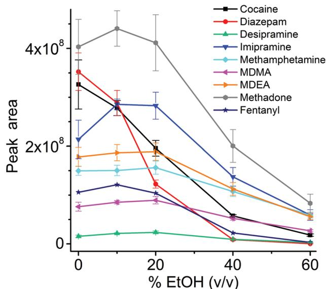
Fig. 5 Extraction efficiency ( $n = 4$ ) for the considered drugs from aqueous solutions at different concentration of EtOH. The ultrasound-assisted extractions were performed in pre-equilibrium (5 min) at 40 °C using  $3 \times 20$  mm thin films immersed in 1.5 mL liquid (in 1.5 mL vials). Each extracted ion chromatogram was integrated for 0.5 min.
