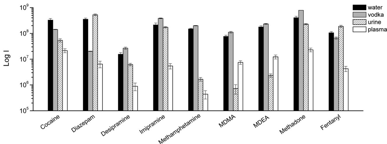
**Fig. 7** TFME-DBDI-MS ion signals for different drugs at  $1 \text{ ng mL}^{-1}$  extracted from vodka, urine, and plasma (1.5 mL, 5 min extraction,  $n = 4$ ).
