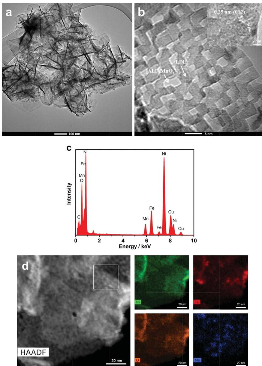
Fig. 4 TEM bright-field micrograph (a), high-resolution (HRTEM) micrograph (b), EDX (c), and HAADF-STEM image and EDX elemental mapping of 10-cycle  $\text{MnO}_x/\text{LDH}$  (d). The white box in (d) indicates the selected region for the HRTEM micrograph in (b).
