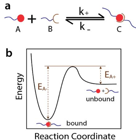
Fig. 2 (a) Reversible crosslinks feature a reversible reaction of functional groups A and B with association rate  $k_+$  and dissociation rate  $k_-$ . (b) Energy landscape of the reversible reaction, with activation energies  $E_{A+}$  and  $E_{A-}$  for the forward and reverse reactions, respectively.
