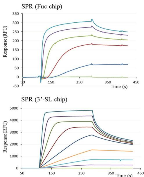
**Fig. 2** SPR sensorgrams obtained by injection of various concentrations of FS-Janus lectin on a fucose chip (upper) with protein concentrations varying between 26 to 312.5 nM and a 3'-sialyllactose chip (lower) with protein concentrations varying between 9.8 nM to 1.25  $\mu\text{M}$ .
