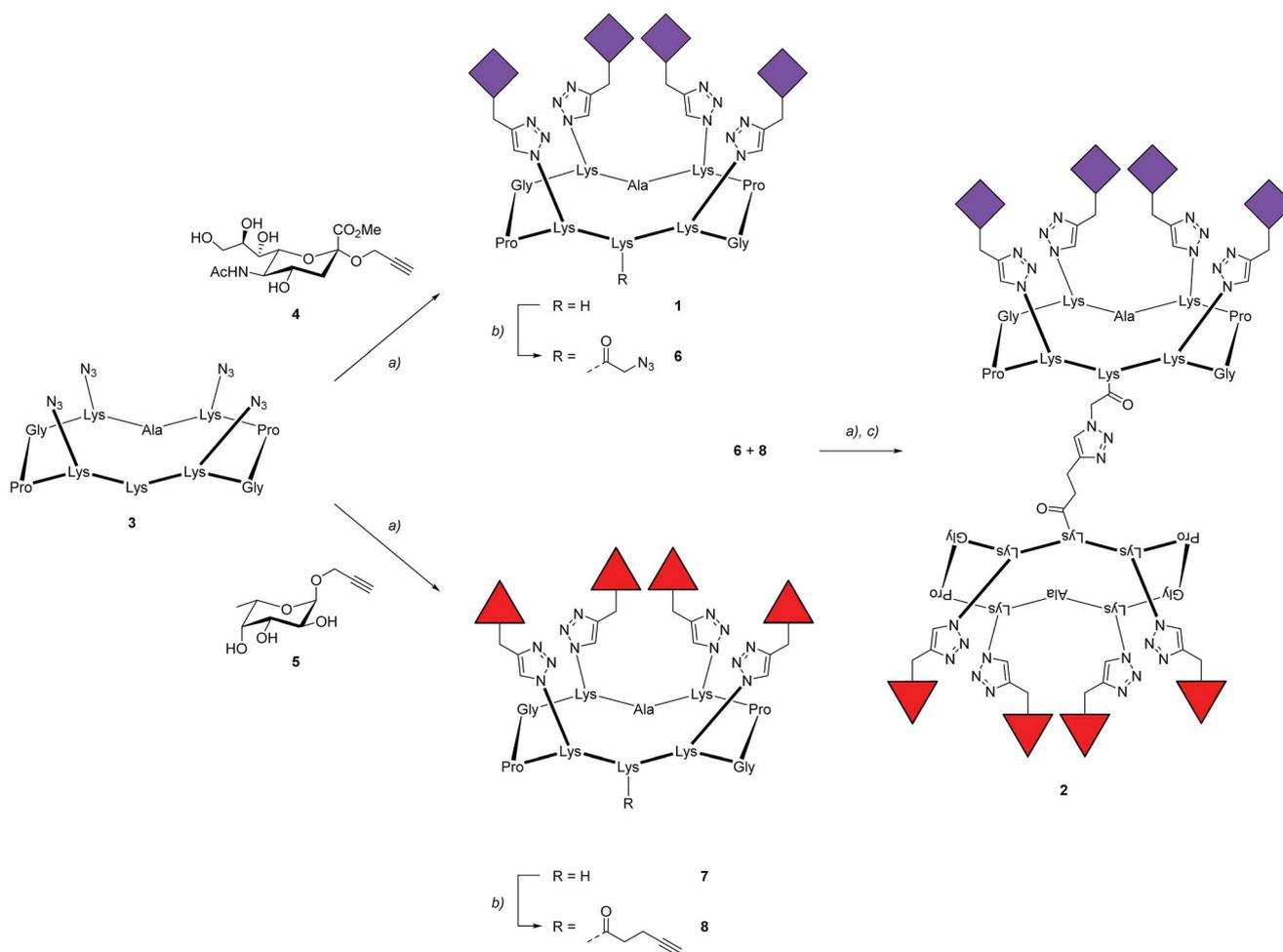
Fig. 3 Synthesis of fucosylated and sialylated glycoclusters. Reagents and conditions: (a)  $\text{CuSO}_4 \cdot 5\text{H}_2\text{O}$ , tris(3-hydroxypropyl)triazolylmethylamine (THPTA), PBS buffer (pH 7.5), r.t., 1 h; (b) *N*-succinimidyl azidoacetate or *N*-succinimidyl pentynoate, DIPEA, DMF, r.t., 2 h; (c) LiOH, r.t., 2 h. All amino acids have the L-configuration.
