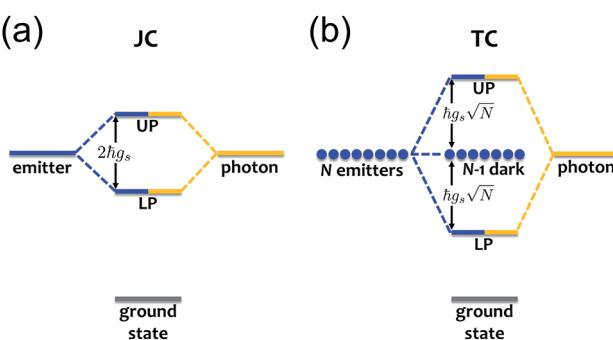
Fig. 2 (a) Jaynes–Cummings (JC) model: emitter and photon strongly couple to form hybridized states termed lower and upper polaritons (LP and UP, respectively) separated in energy by  $2hg_s$ . (b) Tavis–Cummings (TC) model:  $N$  emitters interact strongly with a photon to yield polariton (LP, UP) and  $N - 1$  dark states. The latter do not couple to light and thus maintain the original emitter energy.
