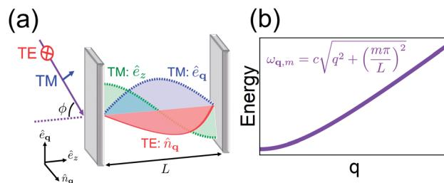
Fig. 1 (a) Representation of microcavity modes excited by radiation (purple) incident at angle  $\phi$ . The electric field polarization of the TE modes (red) lies along  $\hat{n}_q$  while that of TM has  $\hat{e}_q$  (blue) and  $\hat{e}_z$  (green, magnitude only) components. (b) Dispersion (energy as a function of mirror-plane wave vector  $q$ ) of the photonic mode of index  $m$  in microcavity with transverse length  $L$ .
