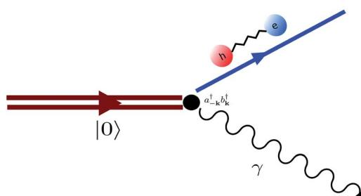
**Fig. 11** Diagram representing spontaneous production of correlated exciton–photon pairs from the bare system ground-state  $|0\rangle$ . This process is significant in the ultrastrong coupling regime where light–matter couplings of the form  $(a_{-k}^\dagger b_k^\dagger + \text{h.c.})$  become relevant (see eqn (15)).
