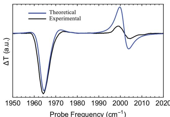
Fig. 9 Experimental and theoretical pump-probe (differential) transmission spectra of strongly coupled  $\text{W}(\text{CO})_6$  in an optical microcavity.<sup>57</sup> These results correspond to the case where the cavity photon and the molecular vibration (asymmetric C=O stretch) are resonant.
