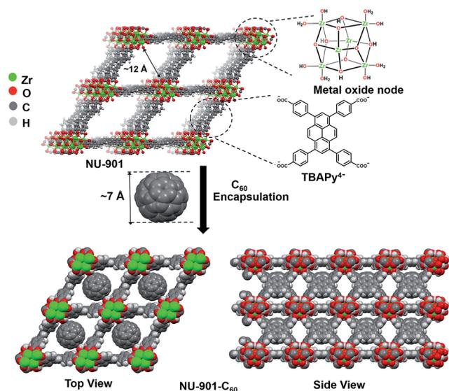
**Fig. 1** Immobilization of  $C_{60}$  within diamond shaped channels of NU-901. The chemical structures of the individual components of NU-901 are shown. The diameter of  $C_{60}$  ( $\sim 7$  Å) is well suited for encapsulation in NU-901 with pore aperture of 12 Å. The top view and side view of the composite NU-901- $C_{60}$  are shown. The top and side views are DFT-optimized structures in the limit of full occupancy of the diamond pores by the fullerene guest, *i.e.* 1 : 1 occupancy.
