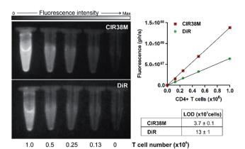
Fig. 5 Determination of the limit of detection in suspensions of CIR38M-labelled and DiR-labelled (both at  $10~\mu\text{M})$  CD4 $^+$  T cells by NIR fluorescence imaging. Values shown as means  $\pm$  s.e.m. Images acquired in PhotonImager<sup>TM</sup> ( $\lambda_{exc.}\sim760$  nm;  $\lambda_{em.}\sim800-900$  nm). Max:  $2\times10^8$  photons per s.
