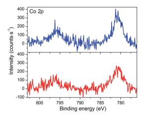
Fig. 4 XPS analyses of the  $NiOlCo_{C11P}$  (blue line) and NiOlRBG-174|Co<sub>C11P</sub> (red line) electrodes at the baseline-corrected Co 2p core level.
