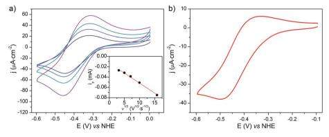
Fig. 8 CVs recorded in a NaCl 0.1 M aqueous electrolyte at (a) a NiO/Co<sub>C11P</sub> electrode at scan rates of 10 (navy line), 25 (blue line), 50 (cyan line) and 100 (purple line) mV s<sup>-1</sup> with (inset) the dependency of baseline-corrected cathodic peak current on the square root of the scan rate (dots) and its linear fit (dashed lines) and (b) a NiOIRBG-174ICo<sub>C11P</sub> electrode at a scan rate of 10 mV s<sup>-1</sup>.
