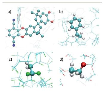
Fig. 2 Illustrations of the atomistic models for the different polymers considered in this study: (a) PIM-1, (b) PS, (c) PVDF, and (d) PEG. A monomer is highlighted in ball-and-stick in each image. Color code: O (red), C (cyan), H (white), N (blue), F (green).
