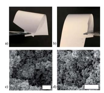
Fig. 7 Comparison of the bulk flexibility of 70 wt% MOF MMMs using PEG (a) and PVDF (b) showing very little difference. Similarly, the SEM microstructure of the PEG (c) and PVDF-based (d) MMMs are very similar. Scale bars are 2  $\mu$ m.
