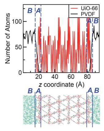
Fig. 5 Top: Atomic density of PVDF (black) and UiO-66 (red) in the direction perpendicular to the surface slab. Note the MOF/polymer overlap in region A. Bottom: Schematic of the interface between PVDF and UiO-66, aligned with the density profile plot.
