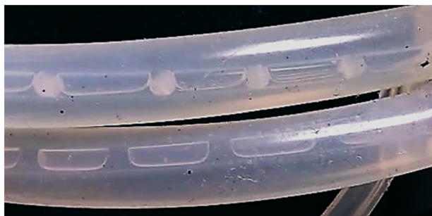
Fig. 5 Image of crystallisation tubing within the cooling tubing jacket at the beginning of the KRAIC. Lower tube is 0.3–0.5 m crystallisation length (32–28 °C), upper tube is 0.9–1.1 m (25–23 °C). N.B. crystals can be seen in solution slugs within the upper tubing.
