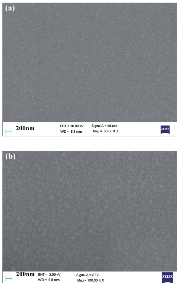
Fig. 4 SEM micrographs of (a) pure PEDOT–PSS thin film (b) PEDOT–PSS thin film doped with 20 wt% EG.
