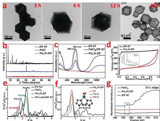
**Fig. 2** (a) The phase change process of Pd<sub>1</sub>/H-ZIF at room temperature, (b) XRD, (c) UV/Vis diffuse reflection spectrum, (d) nitrogen adsorption isotherm and desorption isotherm, (e) the  $k_3$ -weighted  $\chi(k)$ -function of the EXAFS spectra, (f) the corresponding Pd K-edge EXAFS fitting curves of Pd<sub>1</sub>/H-ZIF, and (g) Cl L-edge spectra.
