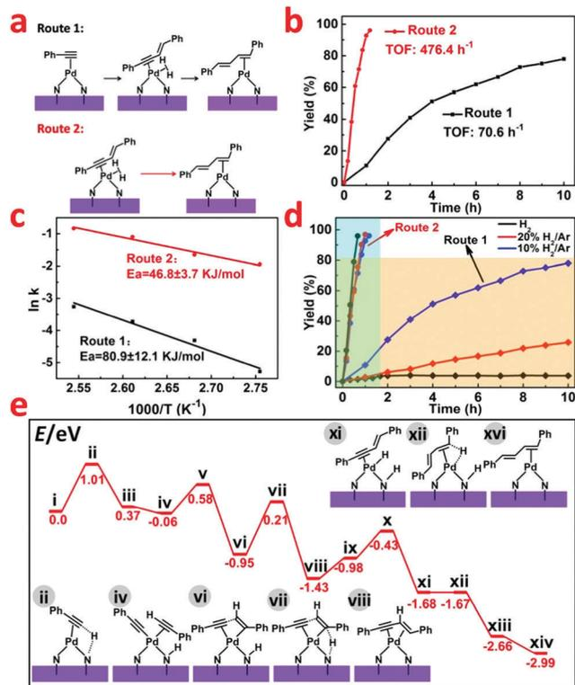
**Fig. 4** (a and b) Different routes in the reaction process. (c) Arrhenius plot of the different reaction routes for Pd<sub>1</sub>/H-ZIF. (d) The influence of different atmospheres in different routes. (e) Energies of intermediates and transition states in the mechanism of phenylacetylene dimerization at the Pd<sub>1</sub>/H-ZIF from DFT calculations.
