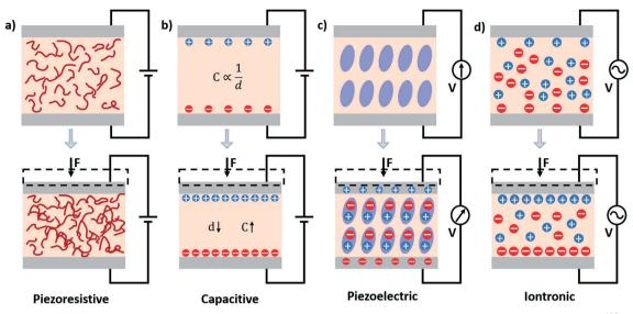
Fig. 5 Schematics illustrating the different modalities of mechanical sensors. a) Piezoresistivity; b) capacitance; c) piezoelectricity; <sup>190</sup> d) iontronic.
