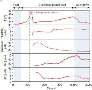
Fig. 17 Bringing electrochemical sensors directly onto skin to detect sweat (adapted). 158 In all the examples provided in the figure, technology is mechanically compliant to skin, which is a first step to reduce the sweat volume between skin and sensors. The data shown in (f) is for a human subject wearing the technology shown in (d). 178
