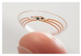
Fig. 19 The contact lens sensor that was under co-development by Google and Novartis (effort ceased) measures glucose concentration in tears using a miniaturized electrochemical glucose sensor and a wireless chip and antenna ring. Copyright 2014, Google X.
