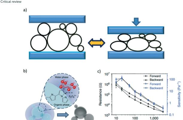
Fig. 8 a) Schematic illustration of the elasticity of hollow sphere structured polypyrrole (PPy). b) Schematic illustration of the phase separation between water and organic components for the synthesis of PPy hydrogels. c) Electrical resistance response to induced pressure.<sup>84</sup>
