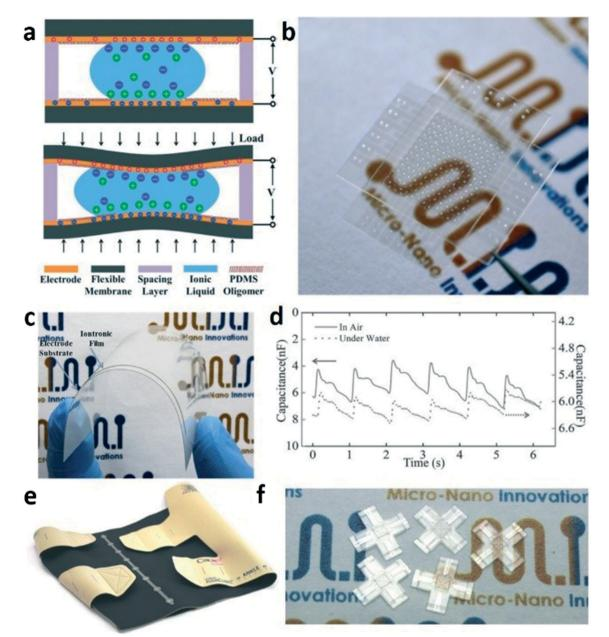
Fig. 10 (a) Iontronic droplet sensor operation principle. (b) Photo of an iontronic microdroplet sensing array. (c) Photo of a flexible ionic gel film on an electrode substrate. (d) Real-time pulse pressure waveforms in dry and underwater environments. (e) Photo of a commercial inelastic legging integrated with the iontronic flexible sensing array. (f) Prototypes of microfluidic tactile sensors for three-dimensional force measurements.
