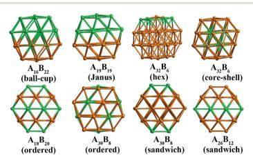
Fig. 2 Examples of 38-TO nanoalloys with different compositions and chemical arrangements. The "hex" configuration has the central atom of one (111) facet surrounded by a hexagon of six atoms of the other element.
