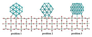
Fig. 3 The three positions studied for 38-TO Pd-Ir and Au-Rh nanoalloy clusters (and their pure metal equivalents) adsorbed on the TiO<sub>2</sub>(110) surface.
