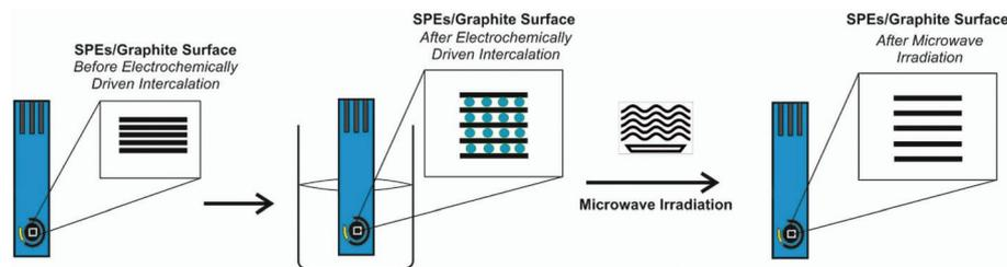
Fig. 1 Schematic overview of the modification protocol of the microwave assisted electrochemically driven intercalated screen-printed electrodes (EDI-SPEs).
