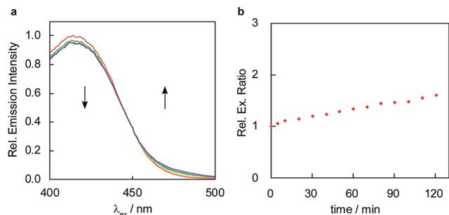
Fig. 1 FA response of RFAP-0. Data were acquired at 37 °C in 20 mM PBS (pH 7.4). Excitation spectra were collected between 400 and 500 nm with emission monitored at  $\lambda_{em} = 510$  nm. (a) Excitation ratiometric response of 10  $\mu$ M RFAP-0 to 100  $\mu$ M FA. Excitation spectra are shown at 0, 30, 60, 90, and 120 min (red, yellow, green, blue, and purple traces, respectively) after the addition of FA. (b) Quantification of 470/420 nm excitation ratio over time.
