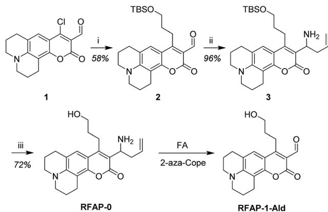
Scheme 2 Synthesis of RFAP-0. Reagents and conditions: (i) lithium bis(3-((*tert*-butyldimethylsilyloxy)propyl)copper, Et<sub>2</sub>O, THF, -20 °C, 3 h; (ii) NH<sub>3</sub>, MeOH, 0 °C, then allylboronic acid pinacol ester, rt, 10 h; (iii) AcOH, H<sub>2</sub>O, rt, 14 h.
