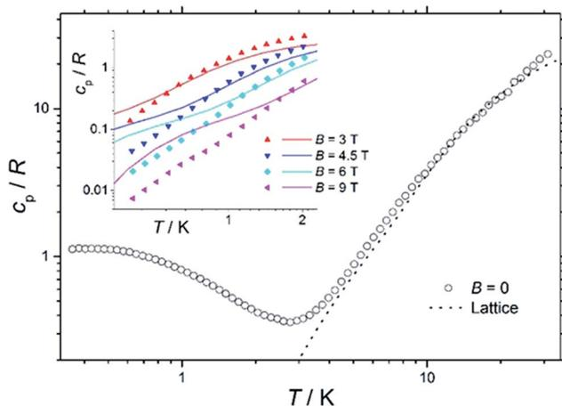
Fig. 7 Temperature dependence of the zero-field heat capacity  $c_p$ , normalised to the gas constant  $R$ , for a polycrystalline sample of **1**. The dotted line is the lattice contribution. Inset: temperature dependence of  $c_p/R$  of **1** for  $T < 2$  K and  $B \geq 3$  T. Solid lines are the best-fit curves, see text for details.
