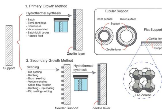
Fig. 3 Schematic of LTA zeolite membrane preparation methods.
