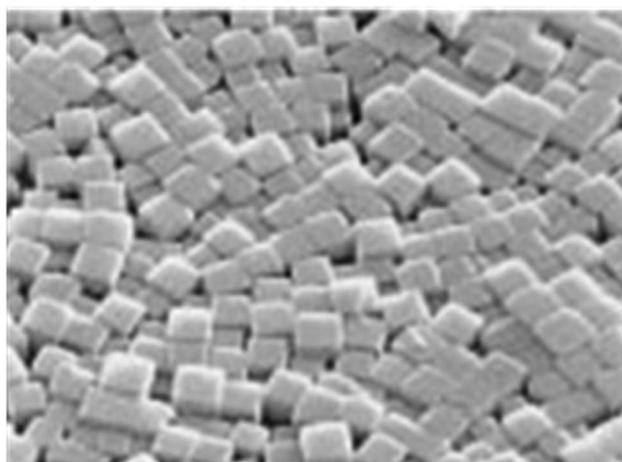
Fig. 2 Typical morphology of LTA zeolite crystal monolayer (magnification  $\times 1200$ ). Reprinted with permission from A. Kulak, Y. J. Lee, Y. S. Park and K. B. Yoon, Orientation-Controlled Monolayer Assembly of Zeolite Crystals on Glass and Mica by Covalent Linkage of Surface-Bound Epoxide and Amine Groups, *Angew. Chem.*, 2000, **112**, 980–983. Copyright (2000) John Wiley and Sons.<sup>72</sup>
