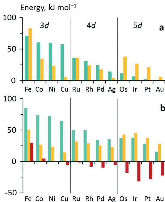
Fig. 7 Energy analyses of the activation energy E_a . (a) Breakdown according to the two-step mechanism: E_a = E_{\text{act}}(\text{OH}) + E'_a for top TSs (bridge TSs for Au and Ag). Color coding: green – E_{\text{act}}(\text{OH}) , yellow – E'_a . (b) Breakdown according to preparation energies for the various parts of the adsorption system, eqn (13): E_a = E_{\text{prp}}(\text{OH}) + E_{\text{prp}}(\text{RCO}) - E_{\text{prp}}(\text{M}) + E_{\text{int}}^{\text{TS}} . Color coding: green – E_{\text{prp}}(\text{OH}) , yellow – E_{\text{prp}}(\text{RCO}) , red – E_{\text{int}}^{\text{TS}} .
