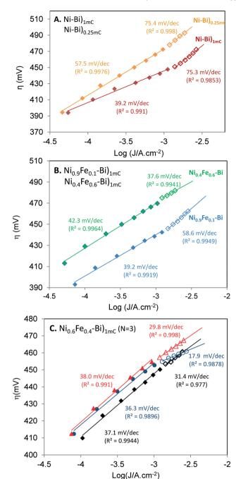
Fig. 5 Tafel plots for Ni–Bi) $_{\rm 1mC}$  and Ni–Bi) $_{\rm 0.25mC}$  (A) and for Ni $_{\rm 0.9}$ Fe $_{\rm 0.1}$ –  $Bi)_{1mC}$  and  $Ni_{0.4}Fe_{0.6}-Bi)_{1mC}$  (B), for films with CVs in Fig. 1 after anodic conditioning. (C) Tafel plots for 3 independently prepared Ni<sub>0.6</sub>Fe<sub>0.4</sub>-Bi)<sub>1mC</sub> anodically-conditioned films. The Tafel slope and the correlation coefficients for the best fit line are shown in the two linear regions.
