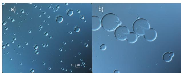
**Fig. 4** (a) Optical micrograph of microcapsules loaded with oleyl alcohol using 1 wt% PVA in water phase. (b) Optical micrograph of typical instability of larger microcapsule where broken and fractured microcapsules are shown with their inner core released out to the surrounding. Scale bar is valid for both micrographs.
