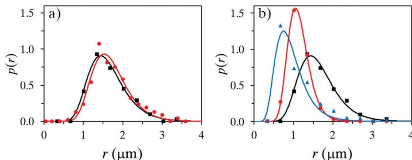
**Fig. 3** (a) Size histograms and fitted lognormal distributions of microcapsules loaded with pure oleyl alcohol using 1 wt% PVA in the water phase (■) compared to using pure water (●). (b) Size histograms and fitted lognormal distributions of the microcapsules (1 wt% PVA) directly after formulation (■), one week after formulation (●), and one month after formulation (▲).
