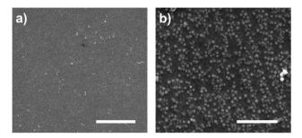
Fig. 5 SEM images of gold surfaces covered with a complete layer of cysteine-tagged Mms6 protein that were patterned by IL at an exposure dose of 100 J cm<sup>-2</sup>, after backfilling with OEG-thiolate and being subjected to a POFHK reaction. Scale bars: a - 10  $\mu m$  and b - 1  $\mu m$ .
