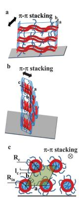
Fig. 6 Models schematically depicting the layer-like structure of thin films of  $P_a$  (a) and  $T_a$  (b). The polymer backbone is represented in red while the film surface is the gray parallelogram. (c) The view along the helical axis represents notations used in eqn (7) and (8). The inner part of the helices is colored in blue, the area of the pseudo-hexagonal unit cell external to the helices is colored in green (c)
