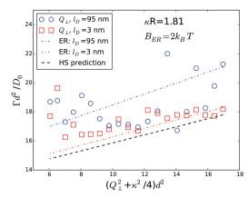
Fig. 10 Normalized initial relaxation rates  $\Gamma$  as a function of the normal scattering vector component squared. Symbols represent experimental data obtained from a  $\phi$  = 0.01 sample at different Debye screening lengths, as indicated in the legend. Lines represent theoretical predictions for infinite dilution according to eqn (5) and (9).
