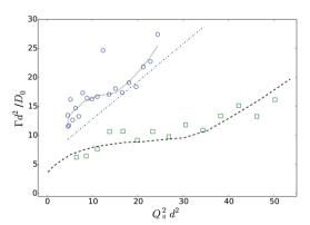
Fig. 12 Comparison of  $Q_{\parallel}$ -scans on a PEGylated FBMA suspension with  $\phi=0.07$  (open circles) and a hard sphere system at  $\phi=0.3$  (open squares). The dashed line represents simulation data for the hard sphere system, the dashed dotted line is the prediction for charged spheres at low  $\phi$  according to eqn (5) and (9) and the dotted line is a guide for the eyes.
