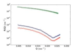
Fig. 6 Static light scattering data at low volume fractions. Open squares:  $\phi$  = 5.6 imes 10<sup>-3</sup> in water, open circles:  $\phi$  = 1.4 imes 10<sup>-3</sup> in DMSO/water, open triangles:  $\phi = 5.6 \times 10^{-3}$  in DMSO/water, lines: best fits to data with eqn (7) resulting the parameters listed in Table 1.
