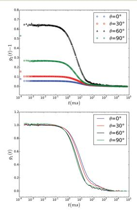
Fig. 2 Time auto correlation functions recorded during a  $Q_{\parallel}$  scan in EWDLS at  $\alpha_{r}=60^{\circ}$  and values of  $\theta$  as indicated in the legend. Top: Intensity correlation functions  $\hat{g}_{2}(t)-1$  as measured. Bottom: Field correlation functions calculated by the generalized Siegert relation, eqn (1).
