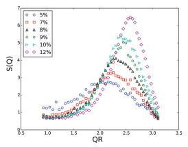
Fig. 7 Structure factors obtained from PEGylated FBMA particle suspensions in index-matching DMSO/water mixtures with different volume fractions as indicated in the legend and a screening length of  $l_{\rm D} \approx 95$  nm.
