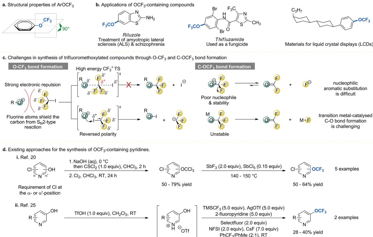
Fig. 1 Properties, applications, synthetic challenges and methods of synthesis of OCF<sub>3</sub>-containing compounds. NFSI = *N*-fluorobenzenesulfonamide, TMSCF<sub>3</sub> = trifluoromethyltrimethylsilane.
