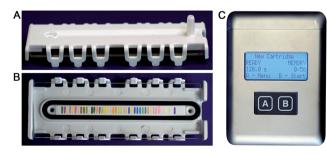
Fig. 1 The optoelectronic nose. (A) The linear array of colorimetric sensors and disposable cartridge. Cartridge side view (7.9  $\times$  2.8  $\times$  1.0 cm). (B) Cartridge front view. (C) Handheld reader/analyzer (12.8 imes 9.5 × 4.0 cm) based on a color contact line imager.
