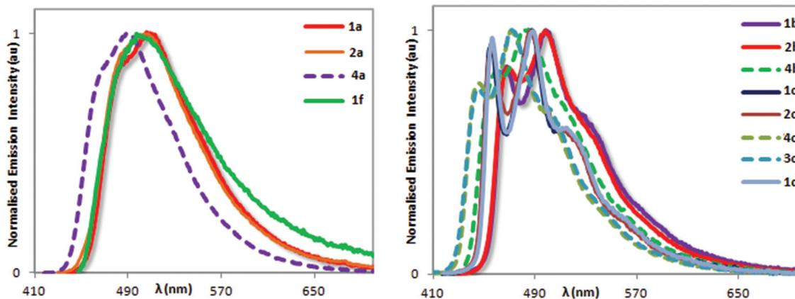
Fig. 4 Normalized photoluminescence spectra of complexes **1a**, **2a**, **4a**, **1f** (a) and **1b**, **2b**, **4b**, **1c**, **2c**, **4c**, **3c**, **1d** (b) recorded in degassed MeCN at 298 K ( $\lambda_{\text{exc}}$ : 360 nm).
