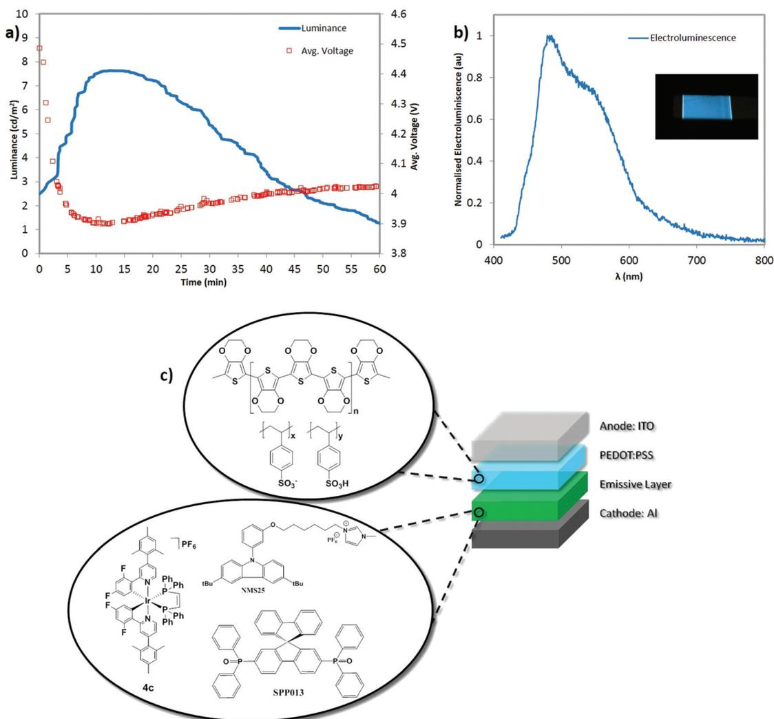
**Fig. 5** (a) Luminance (solid blue line) and average voltage (open red squares) for ITO/PEDOT:PSS/active layer/Al (active layer = 1 : 1 by mass of NMS25 : SPPO13 with 10 wt% of **4c**) with a pulsed driving regime (block-wave pulsed current; 1000 Hz; 50% duty cycle; average density  $100 \text{ A m}^{-2}$ ). (b) Electroluminescence spectrum with inset photo of LEED. (c) Schematic representation of the LEED architecture.
