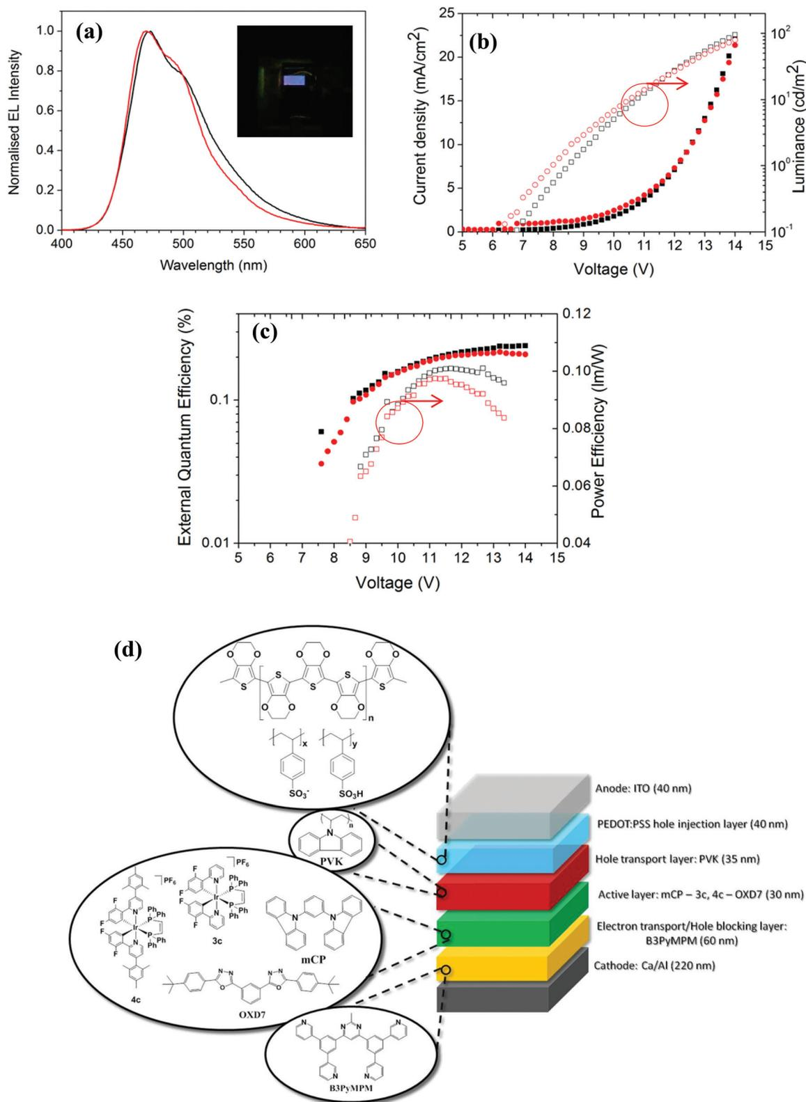
**Fig. 6** (a) Normalized electroluminescent emission spectra of **4c** (black) and **3c** (red) in thin films. Inset shows the photograph of the working OLED with **4c**. (b) Current density and luminance versus applied voltage for OLEDs made with **4c** (black) and **3c** (red). (c) External quantum efficiency and Power efficiency versus applied voltage for OLEDs made with **4c** (black) and **3c** (red). (d) Schematic representation of the OLED architectures.
