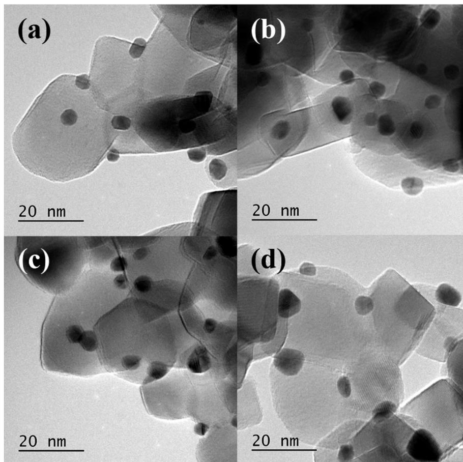
Fig. 6 Representative TEM images of 1% Au/TiO<sub>2</sub> SIM calcined at a) 250 °C, b) 350 °C, c) 450 °C and d) 550 °C.
