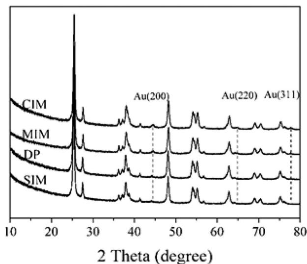
**Fig. 1** XRD pattern of 1% Au/TiO<sub>2</sub> catalysts prepared with different methods.
