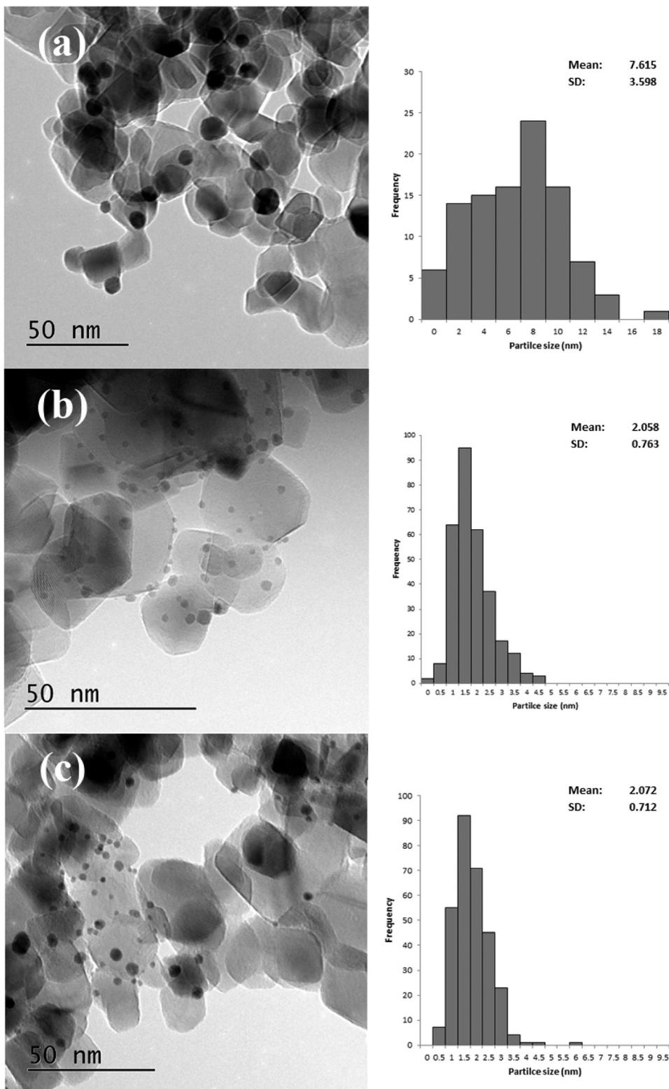
Fig. 9 Representative TEM images and associated particle size distributions for 1% Au/TiO<sub>2</sub> prepared by SIM with different PVA: Au ratios a) 0.1, b) 1.2 and c) 1.8. Particle size distributions based on 300 particles except for a) where 100 particles were counted.
