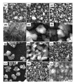
**Fig. 8** SEM images of β-ln<sub>2</sub>S<sub>3</sub> films deposited using the precursors  $[ln(S_2CNCy_2)_3]\cdot 2py$  at (a) 300 °C, (b) 350 °C and (c) 400 °C;  $[ln(S_2CN(Pr)_2)_3]\cdot 1.5py$  at (d) 300 °C, (e) 350 °C and (f) 400 °C;  $[ln(S_2CNPp)_3]\cdot 0.5py$  at (g) 300 °C (h), 350 °C and (i) 400 °C and  $[ln(S_2CNBzMe)_3]$  at (j) 300 °C, (k) 350 °C and (l) 400 °C. Reproduced from ref. 85 with permission from The Royal Society of Chemistry.
