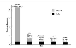
Fig. 37 Maximum gas response of  $In_2O_3$  and  $In_2O_3$ : Ta sensors to different gases in flowing air at optimum operating temperatures. Reproduced with permission from ref. 256. Copyright 2012 American Chemical Society.
