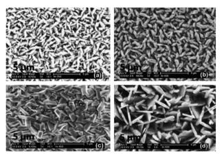
Fig. 7 SEM images of the In<sub>2</sub>Se<sub>3</sub> films deposited from [In(Se<sub>2</sub>P<sup>i</sup>Pr<sub>2</sub>)<sub>3</sub>] at (a) 300 °C, (b) 350 °C, (c) 400 °C and (d) 450 °C. Reproduced with permission from ref. 83. Copyright 2014 Elsevier.
