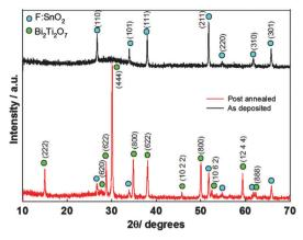
Fig. 34 X-ray diffraction pattern of the as-deposited (black) and post-annealed (red)  ${\rm Bi_2Ti_2O_7}$  thin film. Reproduced with permission from ref. 247. Copyright 2014 Elsevier.
