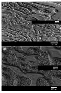
Fig. 5 SEM images of crystalline GaAs films grown via AACVD from As(NMe<sub>2</sub>)<sub>3</sub> and GaMe<sub>3</sub> at (a) 500 °C and (b) 550 °C. Reproduced from ref. 63 with permission from The Royal Society of Chemistry.
