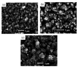
**Fig. 4** SEM images of CdS thin films deposited from [Cd( $S_2$ CNC $_5$ H $_{10}$ ) $_2$ ·py] at (a) 350 °C; (b) 400 °C and (c) 450 °C. Reproduced from ref. 40 with permission from the Centre National de la Recherche Scientifique (CNRS) and the Royal Society of Chemistry.
