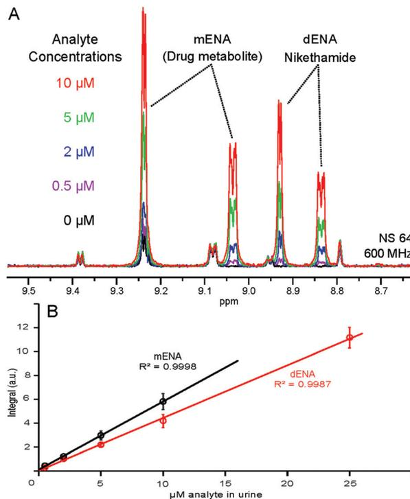
Fig. 5 (A) NMR response at different analyte concentrations; (B) calibration curve for dENA and mENA in urine. Due to the overlap with NA at  $>10 \mu\text{M}$ , mENA calibration was not attempted at higher concentrations. Error bars represent standard errors of three repeated measurements.
