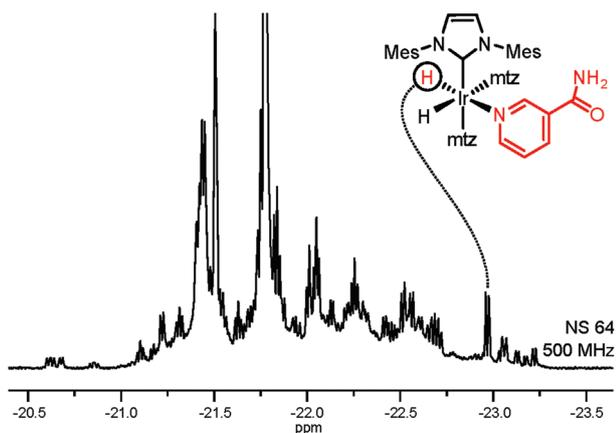
Fig. 2 Hyperpolarized hydride signals of complexes **1** in SPE extract of urine (51%  $p\text{-H}_2$ , 1.2 mM catalyst, 18 mM mtz). The spectrum was acquired using a SEPP pulse scheme (see the ESI†).<sup>20,21</sup>
