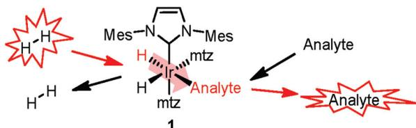
**Scheme 1** Polarization transfer in SABRE. A co-substrate (mtz, 1-methyl-1,2,3-triazole) is introduced for analyte hyperpolarization in the low- $\mu\text{M}$  regime.<sup>11</sup>
