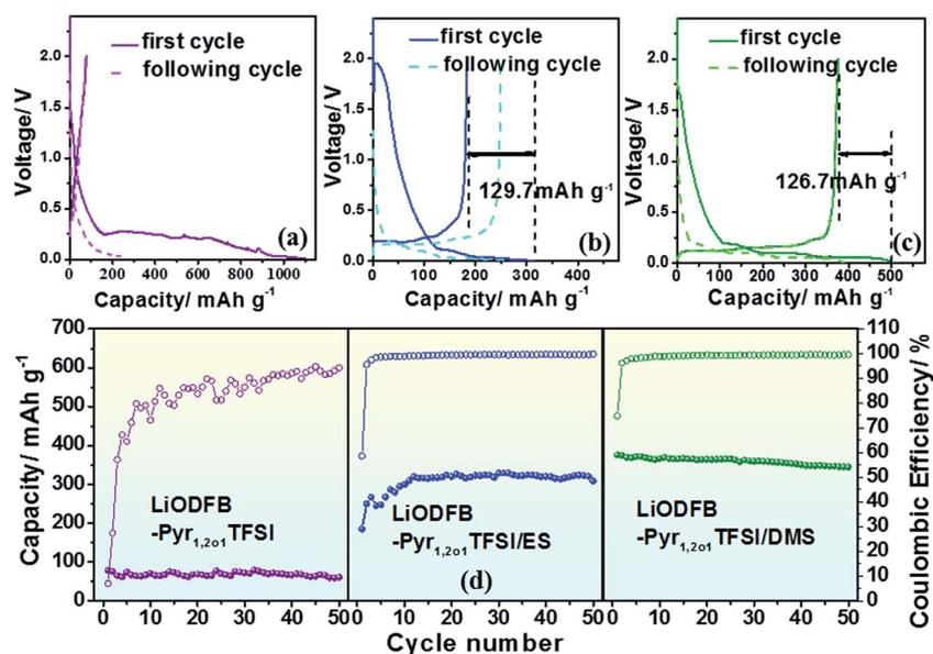
Fig. 3 First and subsequent charge and discharge curves of Li/MCMB cells with (a) LiODFB–Pyr<sub>1,2o1</sub>TFSI, (b) LiODFB–Pyr<sub>1,2o1</sub>TFSI/ES or (c) LiODFB–Pyr<sub>1,2o1</sub>TFSI/DMS electrolytes. (d) Cycling performance and coulombic efficiency of the cells with the three electrolyte samples.
