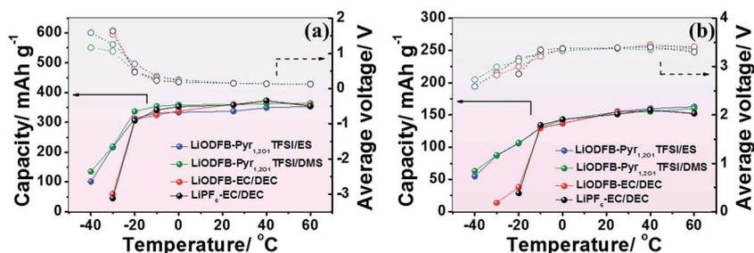
Fig. 6 Performance of Li/MCMB (a) and Li/LiFePO<sub>4</sub> cells (b) containing LiODFB-Pyr<sub>1,2O1</sub>TFSI/ES, LiODFB-Pyr<sub>1,2O1</sub>TFSI/DMS, LiODFB-EC/DEC or LiPF<sub>6</sub>-EC/DEC electrolytes at various temperatures with a current density of 0.1C.
