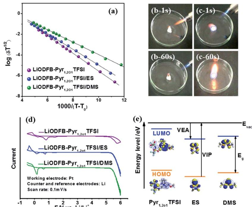
Fig. 2 (a) VTF plots of the conductivity of LiODFB-Pyr<sub>1,2O1</sub>TFSI electrolytes with and without sulphites at various temperatures. Burning tests of (b) LiODFB-Pyr<sub>1,2O1</sub>TFSI/DMS and (c) LiPF<sub>6</sub>-EC/DEC. (d) CVs of LiODFB-Pyr<sub>1,2O1</sub>TFSI electrolytes with and without sulphite. (e) The energy level diagram of frontier molecular orbitals relative to the energy in a vacuum ( $E_{vac}$ ) and HOMO and LUMO plots of Pyr<sub>1,2O1</sub>TFSI, ES and DMS.
