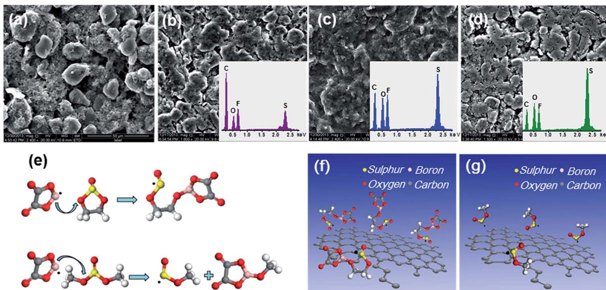
Fig. 5 (a) SEM image of the MCMB anode before cycling. SEM and EDS of the SEI layer on the MCMB anode in (b) LiODFB-Pyr<sub>1,2O1</sub>TFSI, (c) LiODFB-Pyr<sub>1,2O1</sub>TFSI/ES, and (d) LiODFB-Pyr<sub>1,2O1</sub>TFSI/DMS electrolytes after 10 cycles. Schematic illustration of the synthesis route to SEI: (f) ES; (g) DMS, with the prime reactions (e).
