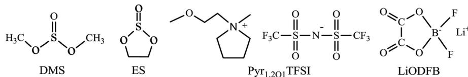
Fig. 1 Molecular structures of the mixture components: dimethyl sulphite (DMS), ethylene sulphite (ES), *N*-methoxyethyl-*N*-methylpyrrolidinium bis(trifluoromethanesulfonyl)-imide (Pyr<sub>1,2O1</sub>TFSI) and lithium difluoro(oxalato)borate (LiODFB).
