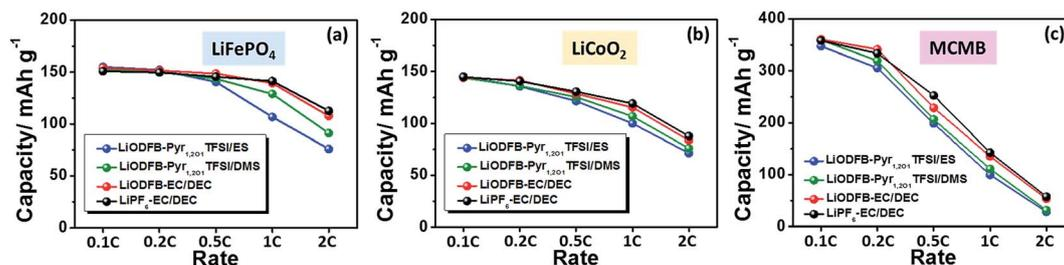
Fig. 7 Rate capability of the Li/LiFePO<sub>4</sub> (a), Li/LiCoO<sub>2</sub> (b) and Li/MCMB (c) cells with LiODFB-Pyr<sub>1,201</sub>TFSI/ES, LiODFB-Pyr<sub>1,201</sub>TFSI/DMS, LiODFB-EC/DEC or LiPF<sub>6</sub>-EC/DEC electrolytes.
