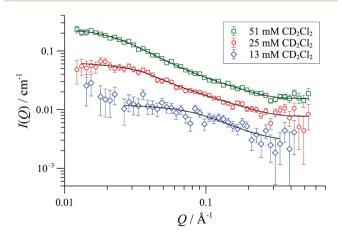
Fig. 11 SANS data and flexible cylinder form factor fits for [1][OTf] in  $CD_2Cl_2$  at 25 °C; fits are for radius 8-9 Å and lengths: 78 Å (13 mM); 156 Å (25 mM) and 332 Å (50 mM).
