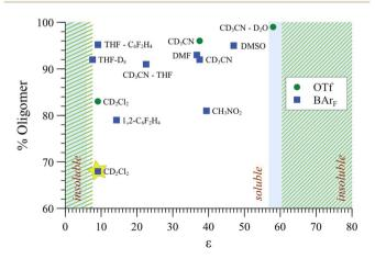
Fig. 9 Oligomerisation ( $^{31}$ P{ $^{1}$ H} NMR, %) of [1][BAr<sub>F</sub>] and [1][OTf] at [Pd]<sub>tot</sub> = 15 mM in solvents of various dielectric constant ( $\varepsilon_r$ ); overlaid areas in green (OTf) and blue (BAr<sub>F</sub>) indicate regions where the complexes are insoluble.
