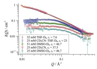
Fig. 10 SANS data and cylinder form factor fits for [1][BAr $_{\rm F}$ ] in various solvents at 25  $^{\circ}$ C.
