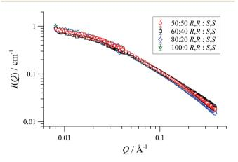
Fig. 3 Fitted SANS profiles and cylinder form factor fits for 32 mM enantio-pure, racemic and scalemic samples of [1][BAr $_{\rm F}$ ] in THF-D $_{\rm 8}$ , 25 °C.
