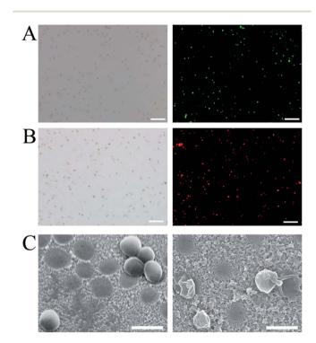
Fig. 5 Optical images of the captured living S. aureus (A) and electrochemically disinfected S. aureus (B) stained by calcein-AM (green) and PI (red) (scale bar = 10  $\mu$ m). (C) SEM images of the captured S. aureus cells before (left) and after (right) electrochemical treatment (scale bar =  $1 \mu m$ ).
