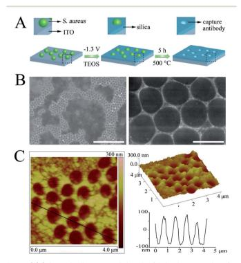
Fig. 1 (A) Schematic diagram outlining the fabrication procedure for the cAbs, (B) SEM micrographs of the cAbs (scale bars = 10  $\mu$ m and 1 μm, respectively), (C) 2D and 3D AFM images, and the corresponding height profiles of the cAbs
