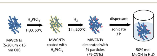
Scheme 1 Synthetic approach for Pt-decorated carbon nanotubes (Pt-CNTs).
