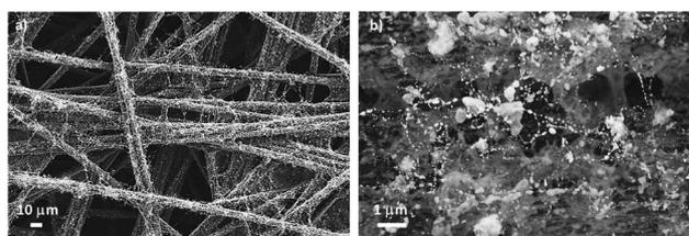
Fig. 5 SEM images of electrospayed 46 wt% Pt-CNT–CsH<sub>2</sub>PO<sub>4</sub> composites, showing direct contact between the electrolyte particles with the carbon nanotubes: (a) low and (b) high magnification.
