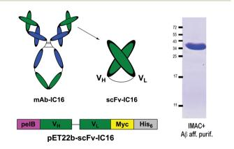
**Fig. 6** Schematic representation of the His<sub>6</sub>-IC16-scFv preparation (left) and purity control after IMAC purification and Aβ-affinity polishing (right).
