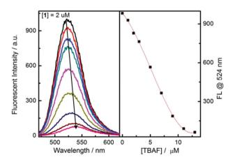
Fig. 5 Fluorescence spectra changes of probe 1 upon addition of TBAF in MeCN.  $\lambda_{ex} = 450$  nm, [1] = 2  $\mu$ M.
