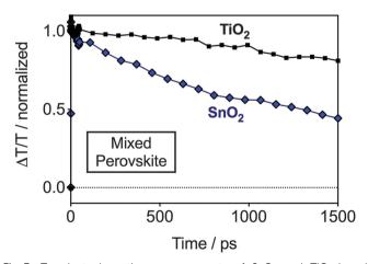
Fig. 3 Transient absorption measurements of  $SnO_2$  and  $TiO_2$ -based planar PSCs. Dynamics of the photo-bleaching bands for photo-excited perovskite measured on a typical working device employing the mixed perovskite (FAPbl<sub>3</sub>)<sub>0.85</sub>(MAPbBr<sub>3</sub>)<sub>0.15</sub> and  $SnO_2$  or  $TiO_2$  as the ESL. The device is held at short circuit condition during the measurement. The probe wavelength is  $\lambda=750$  nm while pumping at  $\lambda=520$  nm.
