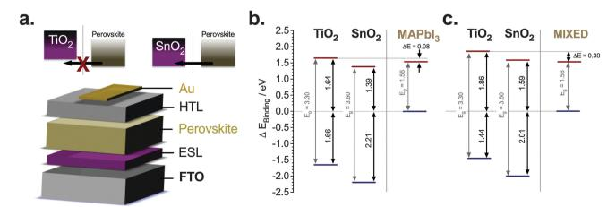
Fig. 1 Energy level diagrams and electron injection characteristics of SnO<sub>2</sub> and TiO<sub>2</sub>-based planar PSCs. (a) Schematic conduction band diagram of the perovskite films and the electron selective layers, TiO2 and SnO2 for (b) MAPbI3 and (c) (FAPbI3)0.85(MAPbBr3)0.15, labeled as 'mixed'
