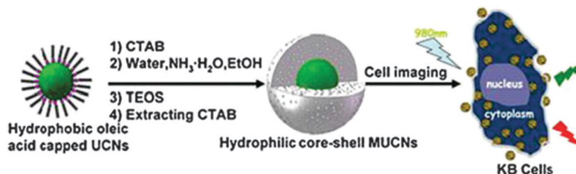
Fig. 8 Schematic of the common method for coating oleate-capped upconversion nanoparticles (UCNPs) with a shell of silica, and their subsequent internalization into cells. From ref. 207 with permission.
