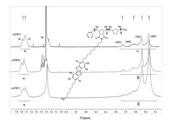
Fig. 1 Key proton peaks of p-BTBT1, 2, and 3
