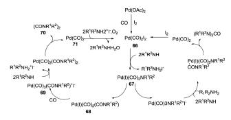
Scheme 82 Proposed reaction mechanism for the oxamide synthesis.
